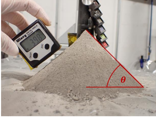
Fig. 2: TRIDENT cuttings pile from drilling to full 1 m depth in NU-LHT-2M. Angle of repose is measured with a digital angle gauge to be 39.8 degrees.
